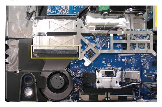
3. Connect the temperature sensor cable and the fan cable to the logic board.
